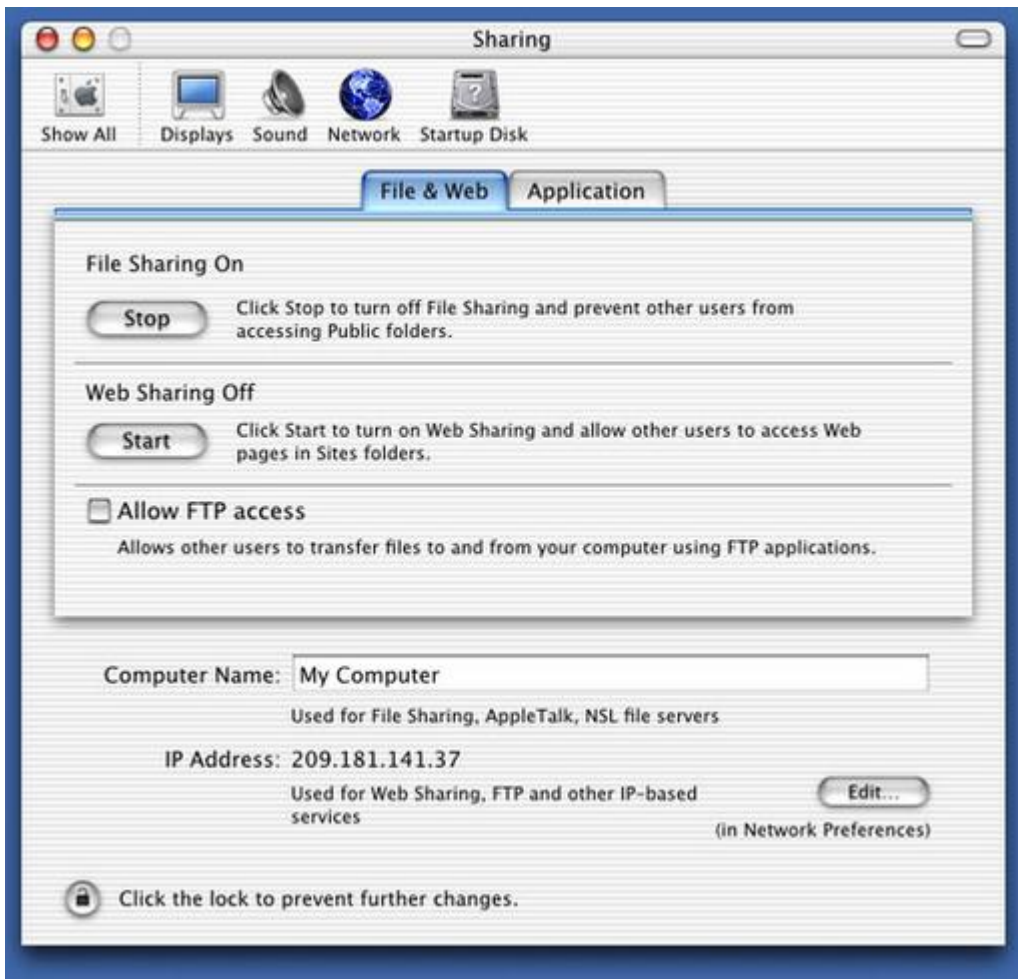
This System Preferences panel allows one to turn on and off Apache and FTP access
